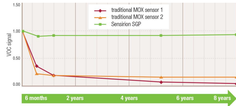
Figure: Long-term stability of the SGP in an accelerated life-time test. The sensors are operated for 200h in 250 ppm D5 (decamethylcyclopentasiloxane) to simulate 10 years of operation in a typical indoor environment.
