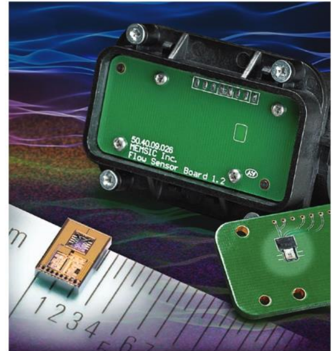
Fig. 1: The MFA1100R thermal gas-flow sensor module integrates the sensing element with on-chip signal-processing and software on a monolithic CMOS process.
